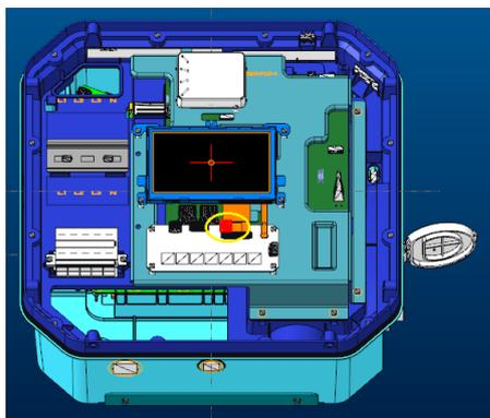
9. Insert nano-SIM card to the SIM socket. (Optional)
