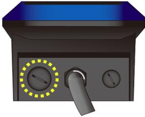
2. Take the provided cable gland and insert the power cable through the gland.
