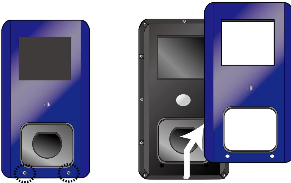
3. Unscrew the fixing 4 screws located around the inner cover.
