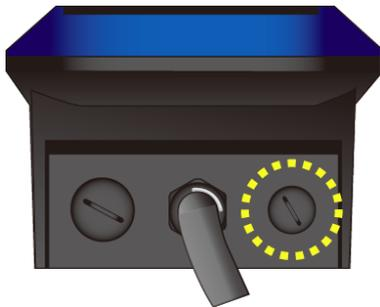
1. Use a big coin to unscrew the cable hole plug.
